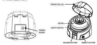
This micro centrifuge is supplied in a packaging box. Open the box, then gently remove the centrifuge from the box and plug in the power adaptor pin before connecting to the main power source. The instruction manual and the accessories should be kept with the centrifuge. Please keep all packaging in safe storage for at least 2 years for warranty purposes.
