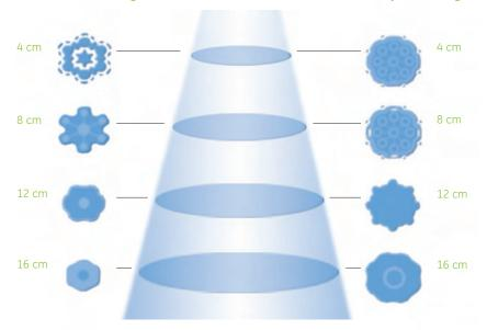
At greater depths, a conventional 7-crystal transducer has a narrower focal region.
