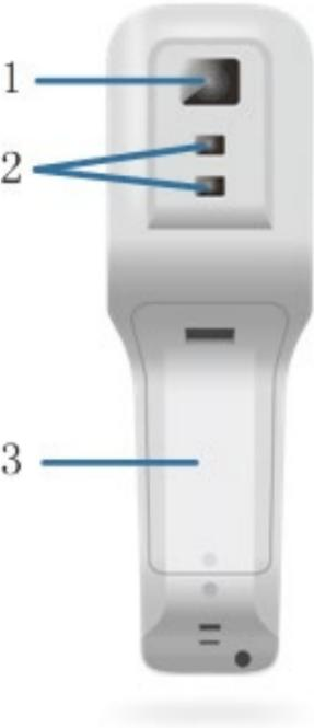
1–Projection window: Used to receive infrared light and project an image.
