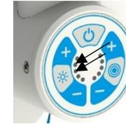
Flashing LED 2 and LED 3 – pairing mode activated
