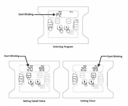
Speed and time value for that particular program is now saved. Press the "Start Button" to start the program mode operation. Once set RPM is reached, the program "Px" (with x = 1 to 9) and its "Speed" & "Time" value will display alternatively.
