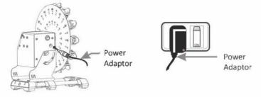
After connecting the power adaptor to back side of the device, switch the main power supply to "ON" & then switch the device on from the rear. Make sure that tubes are loaded properly before use.
