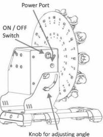
nob for adjusting angle of the disc plate
