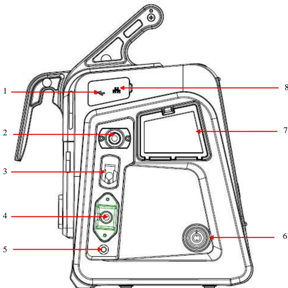
1. USB port: the ventilator software can be upgraded through the USB port, and configuration information, trend data, screenshots, log and calibration forms can also be exported through the USB port.
