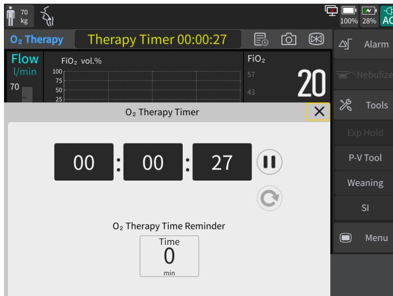
Touch or key to stop or start the timer. Touch the key to reset the displayed time to zero. Set the remaining time in [O<sub>2</sub> Therapy Time Reminder]. When the scheduled time is up, a prompt tone will be issued by the system and the oxygen supply will not be interrupted at this time.
