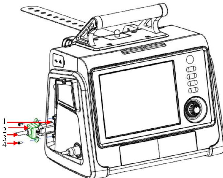
1. AC power socket      2. Socket limiting base      3. AC power cord      4. Screws
