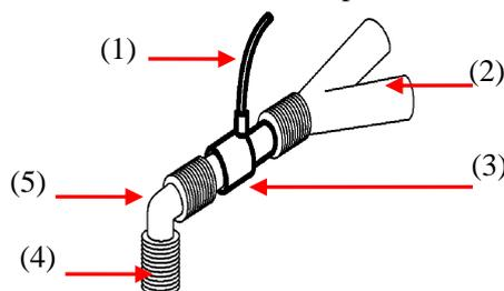
(1) Sampling line (2) Y-shaped tube (3) Airway adapter (4) Breathing tube port (5) Elbow tube
