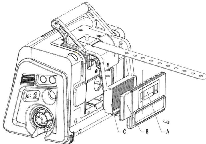
A. Air inlet dust filter                      B. High-efficiency filter cover                      C. HEPA high-efficiency filter
