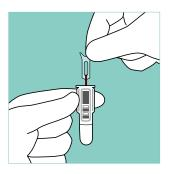
Insert the sample collector into the cuvette within 2 minutes.
