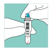
Close the cuvette tightly with the easy CRP reagent cap. Do not press down the turquoise inner part of the reagent cap. Perform the test within 2 hours.
