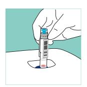
Choose Measure on the display of the QuikRead go instrument. Insert the cuvette in to the measurement well of the instrument. The barcode should be facing you.
